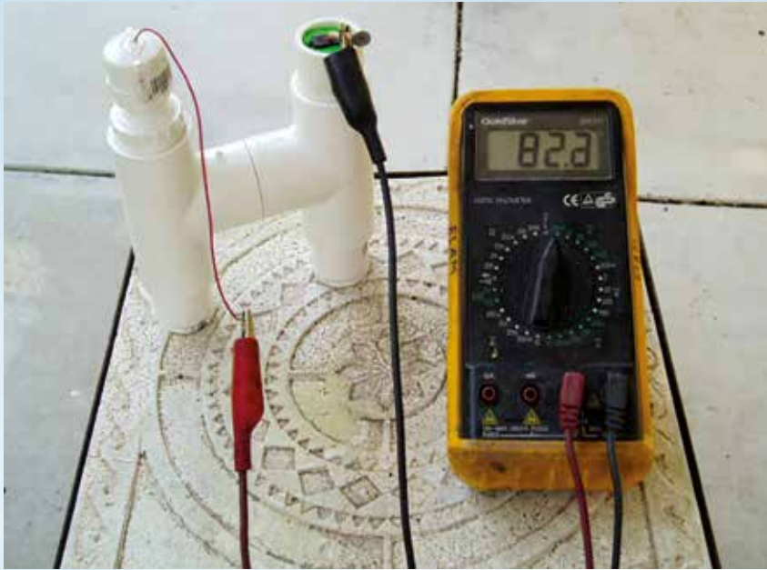
Gene Snider's two-chamber MFC with a salt bridge
